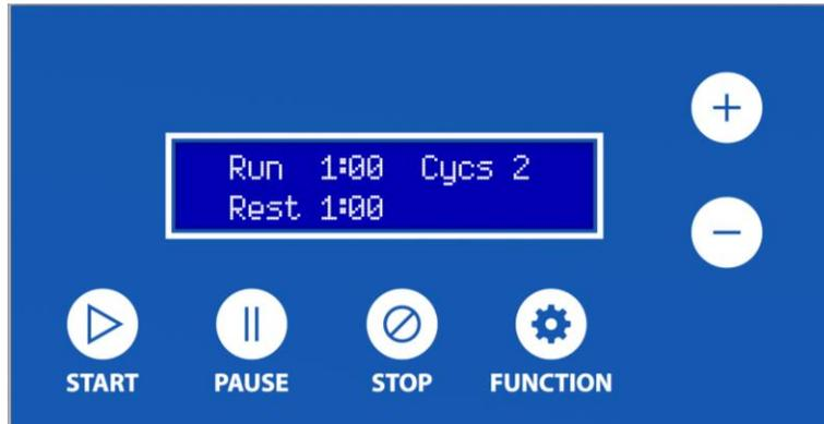
**Figure 2** – BM-400/BM-450 Mixer/Mill Digital Timer Screen and Controls
